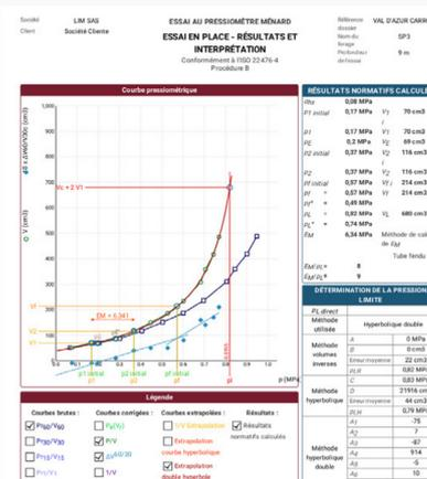
BOR pressuremeter datafiles are then transmitted over the internet from **PocketLIM 5G** with **LIM@mail** service. Pressuremeter data is automatically processed and analysed according to EN ISO 22476 standard to obtain PDF of each pressuremeter test report and corrected curve.
