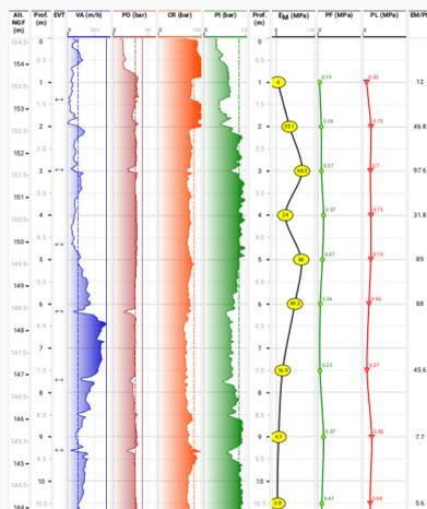
Pressuremeter borehole log
